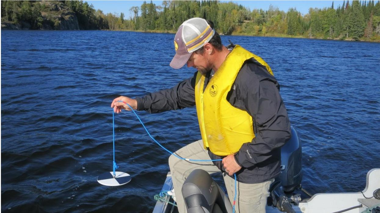
Figure 2 – Lowering of Secchi disk
