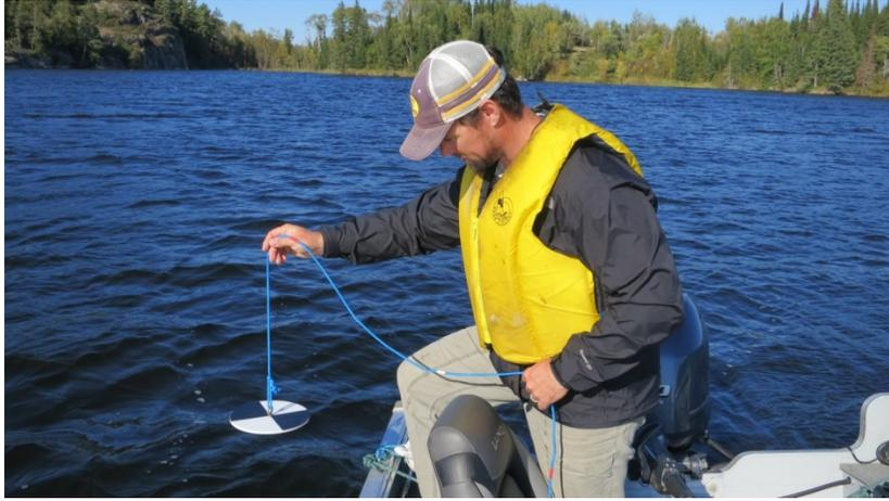
Figure 2 – Lowering of Secchi disk
