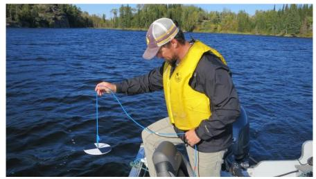
Figure 2 – Lowering of Secchi disk
