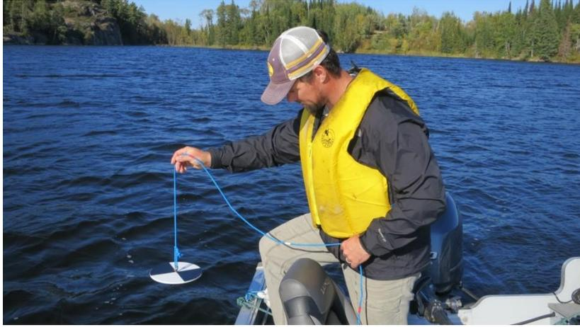
Figure 2 – Lowering of Secchi disk
