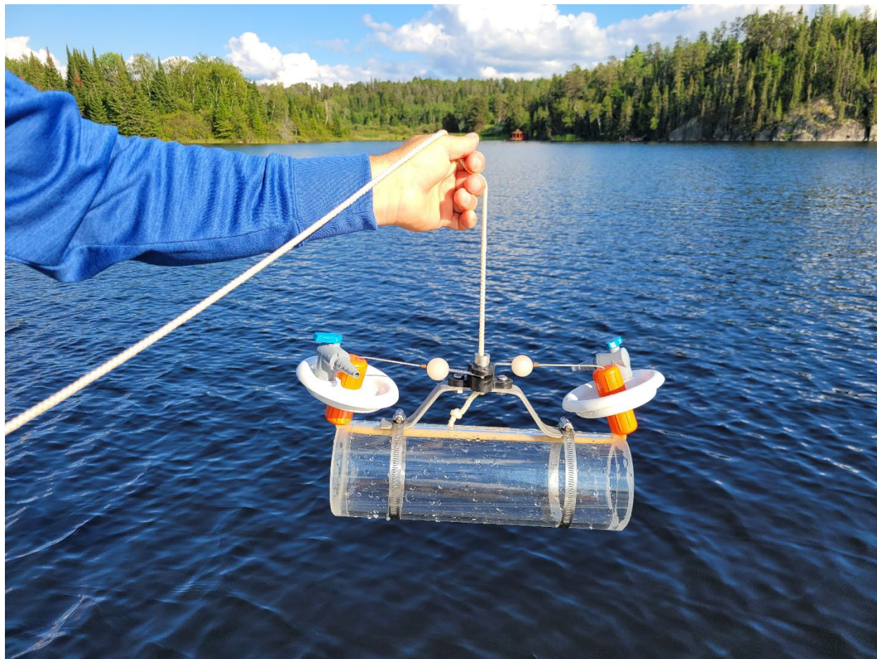
Figure 5 – Horizontal Beta Sampler prior to deployment
