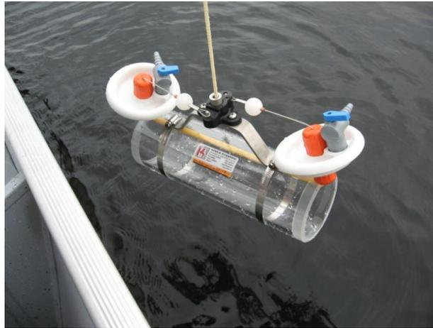
Figure 4 – Horizontal Beta Sampler prior to deployment
