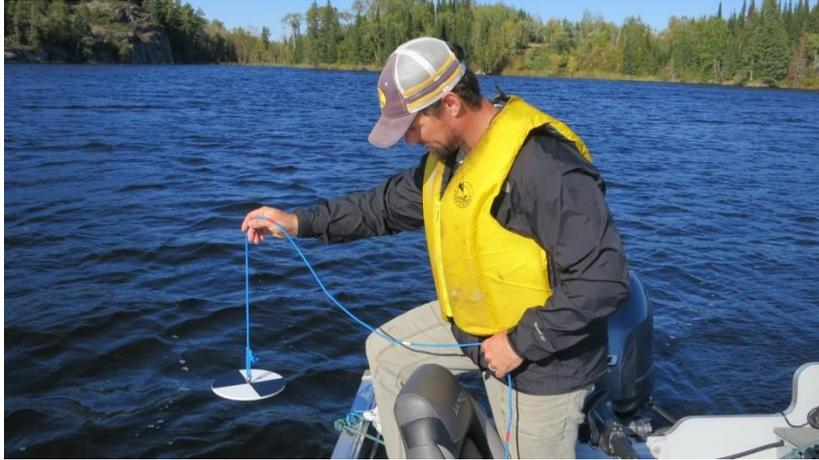
Figure 2 – Lowering of Secchi disk
